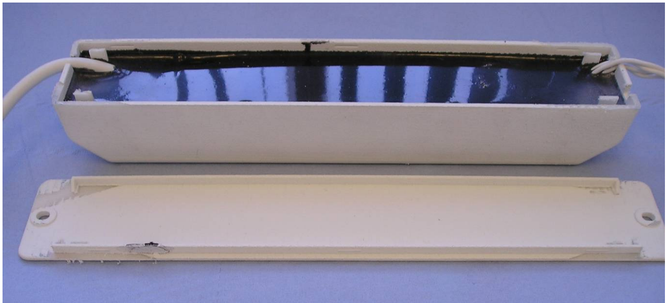
Base plate removed to show potted enclosure
